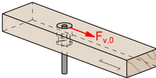
$\alpha = 90^\circ$  (load direction perpendicular to the grain)
