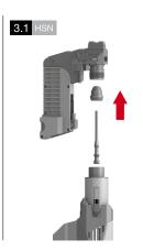
Change if either the Piston or Piston Brake is worn. Change only as a set both Piston and Piston Brake.
